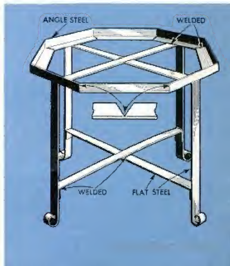
Illustration above shows tile being checked for proper clearance in steel-angle table frame. Hexagonal frame and base were made as in the detail below
